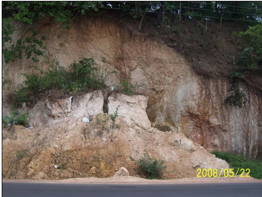
Photo 121: The plan view of the debris slump with steep unstable crown
