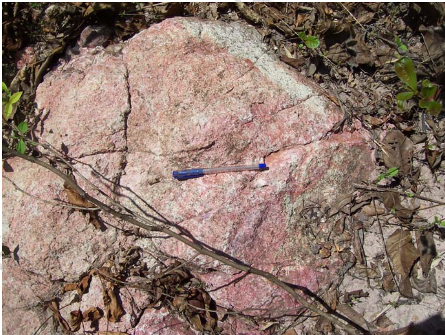
Photo 93: The kaolinised clay lenses in the surface of the debris slide
