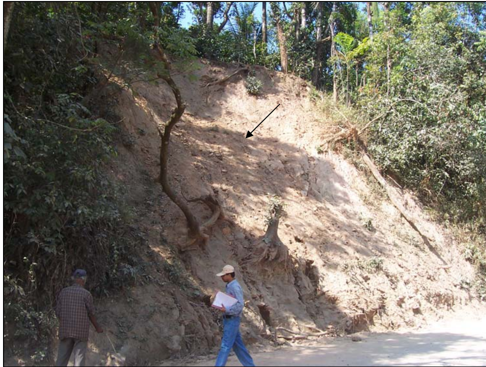
Photo 15: Shallow debris slide with a concave sliding plane
