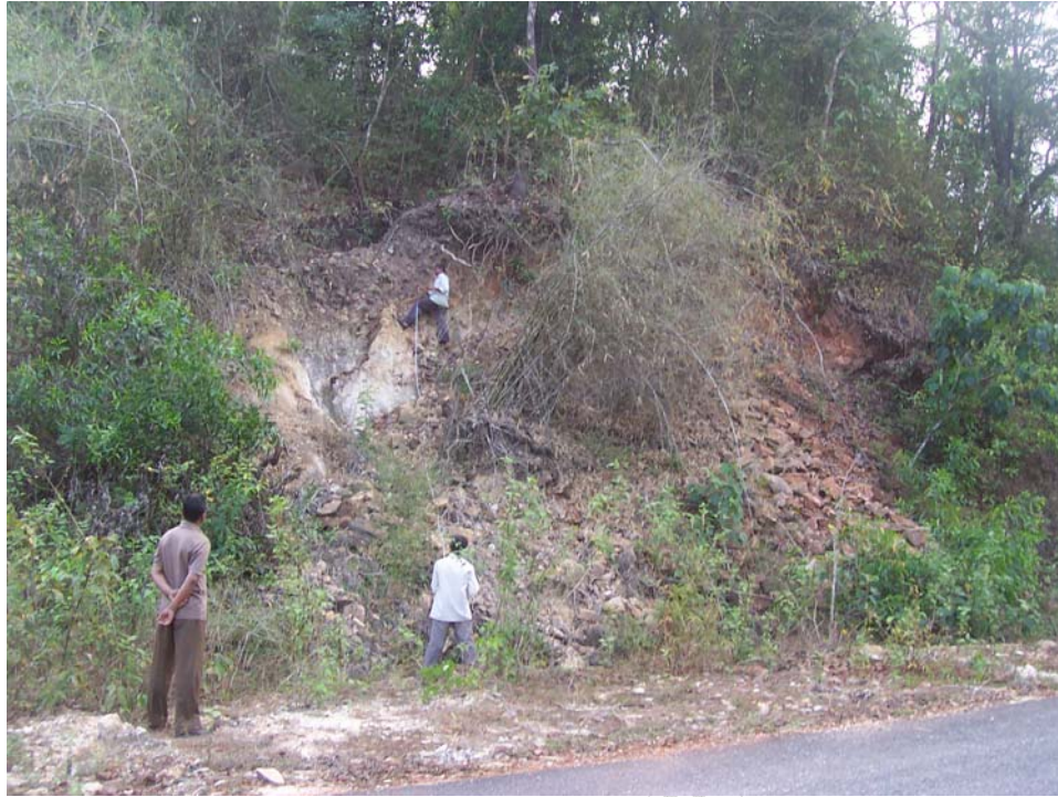
Photo 58: The plan view of the rock slide in a planar failure
