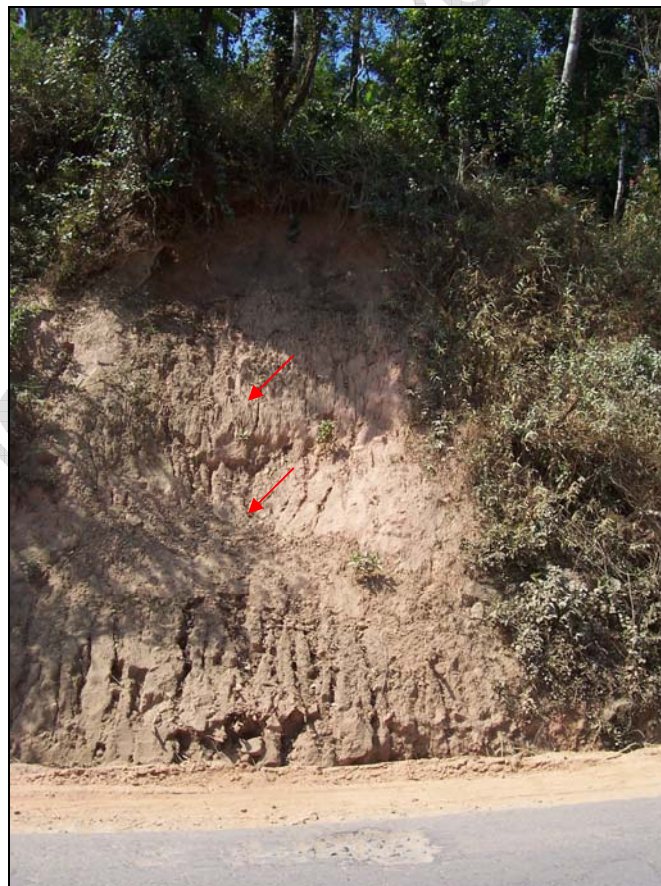
Photo 18: The concavity and convexity of the slide plane.
