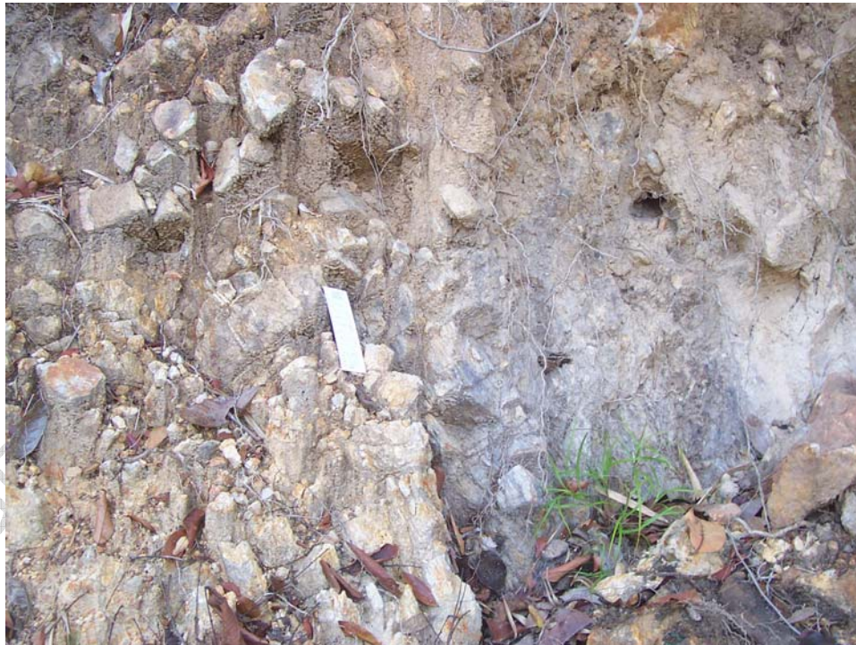
Photo59: The biotite gneiss exposed in the failure plane
